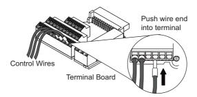
Figure 3.24 Terminal Board Wiring Guide
