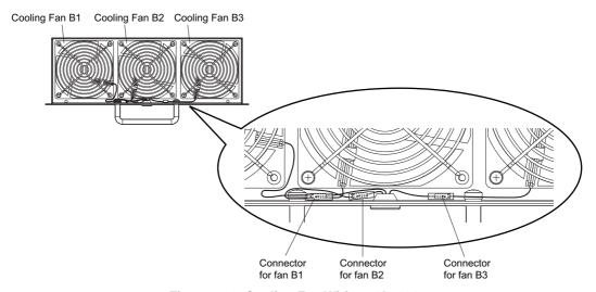
Figure 7.30 Cooling Fan Wiring: 4A0414
