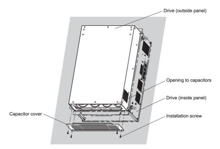
Figure D.10 Capacitor Cover
