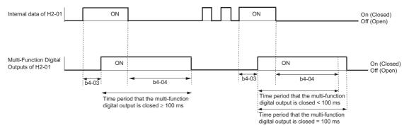
**Note:** Even if the length of the off-delay time and on-delay time for multi-function digital output are each less than 100 ms, the multi-function digital output closes for at least 100 ms.
