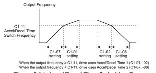
Figure 5.34 Accel/Decel Time Switching Frequency
