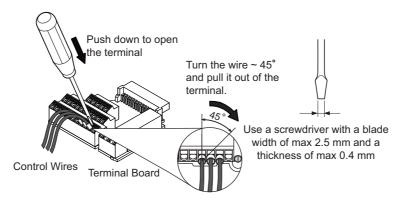
Figure 3.25 Removing Wires from the Terminal Board
