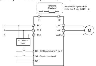
Figure 5.100 KEB Function Wiring Example
