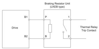
Figure 8.19 Connecting a Braking Resistor Unit: LKEB Type (CIMR-A□2A0004 to 2A0138, 4A0002 to 4A0072)
