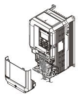
Figure 7.57 Drive Replacement: Removing the Terminal Cover
