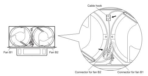
Figure 7.24 Cooling Fan Wiring: 2A0250, 2A0312 and 4A0208
