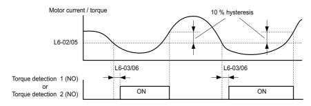
Figure 5.107 Undertorque Detection Operation
