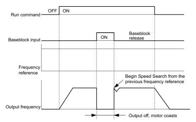
Figure 5.60 Baseblock Operation During Run
