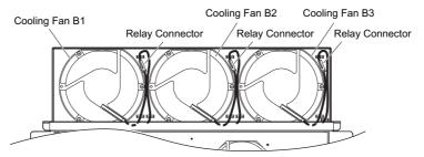
Figure 7.36 Cooling Fan Wiring: 4A0515 and 4A0675
