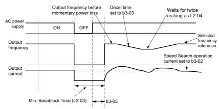
Figure 5.20 Current Detection Speed Search after Power Loss
