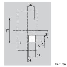
Figure 2.12 Panel Cut-Out Dimensions (External/Face-Mount Installation)
