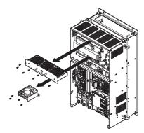
Figure 7.28 Removing the Fan Unit: 4A0414
