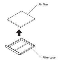
Figure 7.55 Air Filter Replacement: Taking Out the Filter
