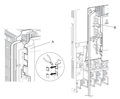
A – Route wires through the openings provided on the left side of the front cover. </>
