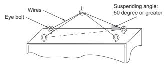
Figure 2.8 State of Suspension with Wires
