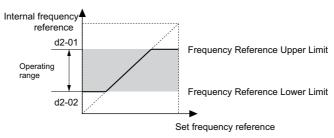
Figure 5.46 Frequency Reference: Upper and Lower Limits
