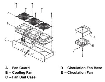
Figure 7.29 Fan Unit Disassembly: 4A0414
