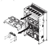
Figure 7.34 Removing the Fan Units: 4A0515 and 4A0675
