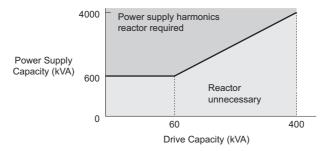
Figure i.1 Installing a Reactor
