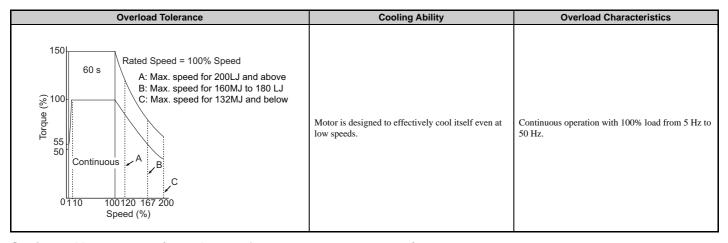
Setting 3: Vector motor (speed range for constant torque: 1:100)
