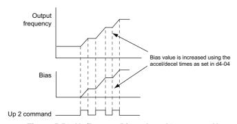
Figure 5.51 Up/Down 2 Bias when d4-03 = 0.00 Hz
