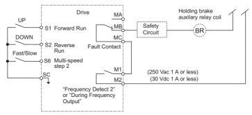
Figure 4.13 Sequence Circuit Configuration
