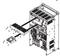
Figure 7.31 Installing the Cooling Fan Unit: 4A0414
