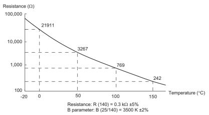
Figure 5.94 Temperature and Resistance of NTC Thermistor
