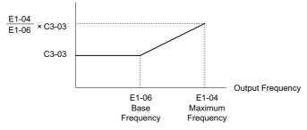
Figure 5.36 Slip Compensation Limit
