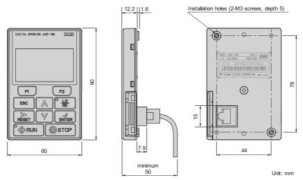
Figure 2.10 Digital Operator Dimensions
