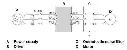
Figure 8.28 Output-Side Noise Filter
