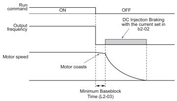
Figure 5.7 DC Injection Braking to Stop
