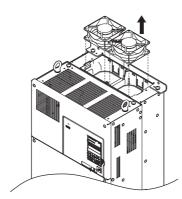
Figure 7.15 Removing the Cooling Fan: 4A0088 and 4A0103
