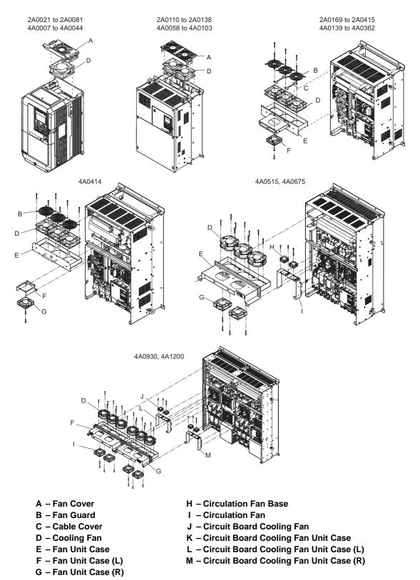
Figure 7.2 Cooling Fan Component Names
