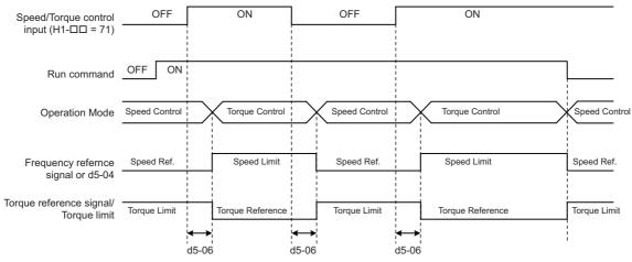
Figure 5.54 Speed/Torque Control Switching Time
