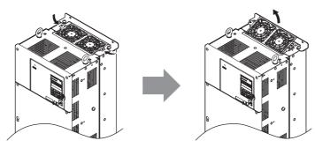
Figure 7.8 Removing the Cooling Fan Cover: 2A0110 and 2A0138, 4A0058 and 4A0072
