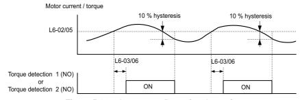
Figure 5.106 Overtorque Detection Operation
