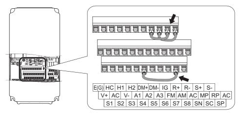
Figure C.8 Terminal Connections for Communication Self-Diagnostics
