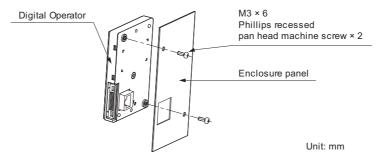
Figure 2.11 External/Face-Mount Installation
