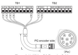
Figure 8.11 Wiring PG Encoder Cable
