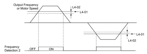
Figure 5.73 Frequency Detection 2 Time Chart
