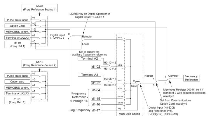
Figure 5.44 Frequency Reference Setting Hierarchy
