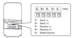
Figure C.2 Serial Communications Cable Connection Terminals (TB4)
