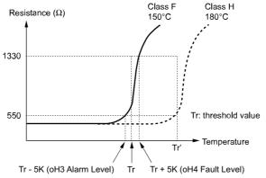
Figure 5.92 Motor PTC Characteristics
