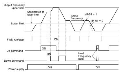
Figure 5.61 Up/Down Command Operation
