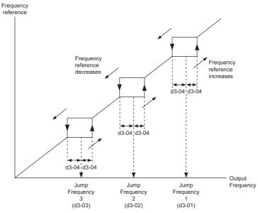
Figure 5.47 Jump Frequency Operation
