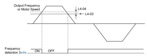
Figure 5.76 Frequency Detection 3 Example with a Positive L3-04 Value
