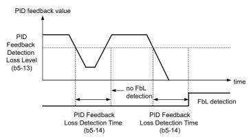
Figure 5.27 PID Feedback Loss Detection
