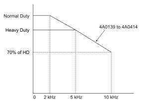
Figure A.4 Carrier Frequency Derating (CIMR-A□4A0139 to 4A0414)
