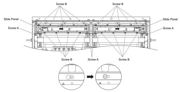
Figure 7.43 Removing the Fan Unit: 4A0930 and 4A1200
