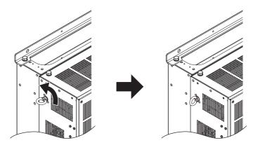
Figure 2.6 Adjusting Angle of Eye Bolts (CIMR-A□2A0360, 2A0415, 4A0250 to 4A0675)
