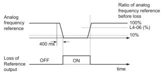
Figure 5.105 Loss of Reference Function
