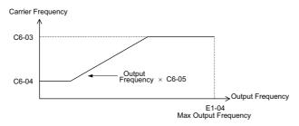
Figure 5.43 Carrier Frequency Changes Relative to Output Frequency
