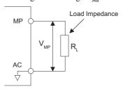
Figure 3.28 Pulse Output Connection Using Internal Voltage Supply
