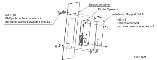
Figure 2.13 Internal/Flush Mount Installation
