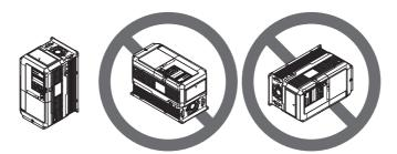
Figure 2.1 Correct Installation Orientation
