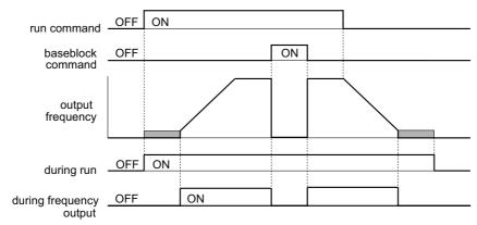
Figure 5.79 During Frequency Output Time Chart
