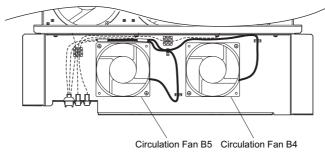
Figure 7.38 Cooling Fan Wiring: 4A0515 and 4A0675
