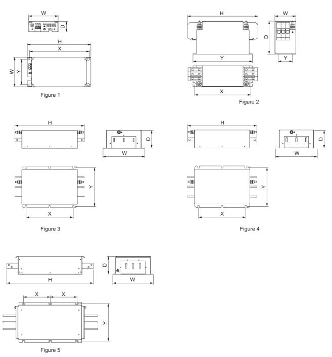
Figure D.7 EMC Filter Dimensions (Manufacturer: Block)
