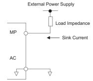
Figure 3.29 Pulse Output Connection Using External Voltage Supply
