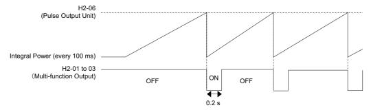
Figure 5.80 Watt Hour Output Example
