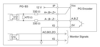
Figure 8.10 Open-Collector Outputs for the Interface Circuit
