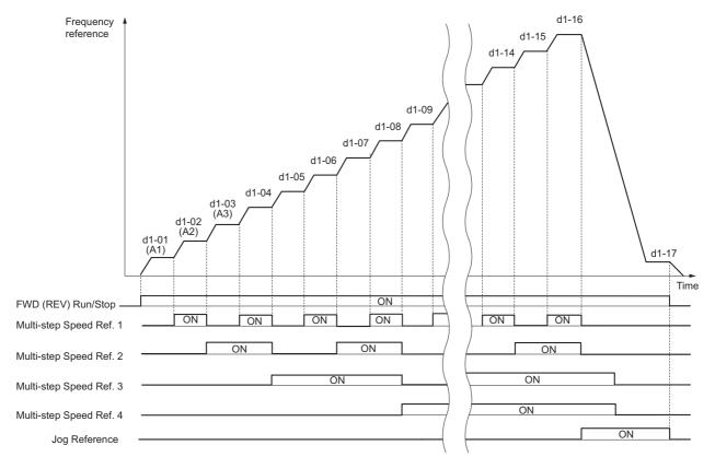
Figure 5.45 Preset Reference Timing Diagram
