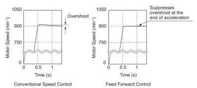
Figure 5.110 Overshoot Suppression by Feed Forward Control
