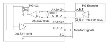
Figure 8.13 Interface Circuit (PG-X3)
