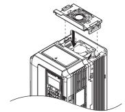
Figure 7.7 Reattach the Fan Cover: 2A0021 to 2A0081, 4A0007 to 4A0044
