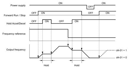
Figure 5.48 Frequency Reference Hold with Accel/Decel Hold Function
