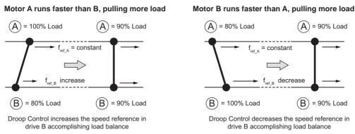
Figure 5.30 Droop Control in a Traverse Application
