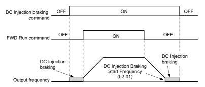
Figure 5.67 DC Injection Braking Input Timing Diagram
