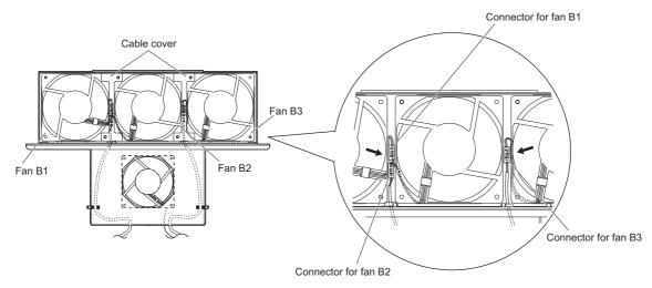
Figure 7.25 Cooling Fan Wiring: 2A0360, 2A0415, 4A0250 to 4A0362
