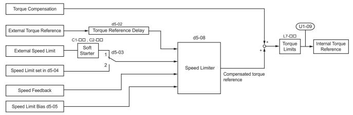
Figure 5.53 Torque Control Block Diagram
