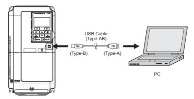
Figure 3.30 Connecting to a PC (USB)
