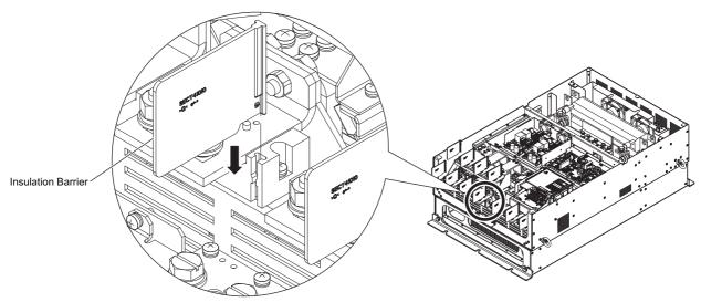
Figure 3.19 Installing insulation barriers
