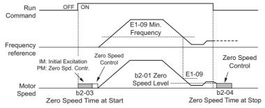
Figure 5.12 Run at the Frequency Reference
