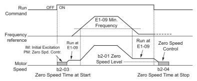
Figure 5.14 Run at the Minimum Frequency
