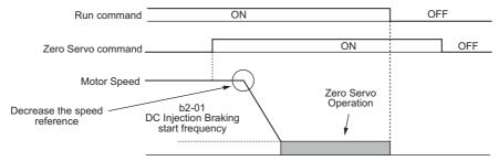
Figure 5.32 Zero Servo Operation
