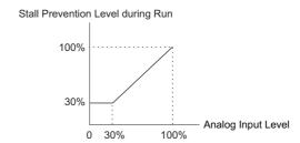
Figure 5.85 Stall Prevention During Run Using an Analog Input Terminal
