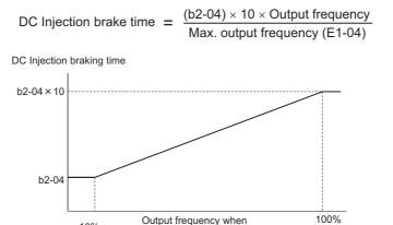
Figure 5.8 DC Injection Braking Time Depending on Output Frequency
