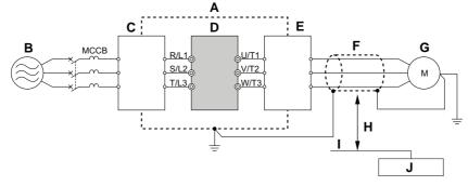
A - Metal enclosure F - Shielded motor cable
