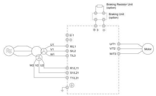
Figure 3.3 Connecting Main Circuit Terminals
