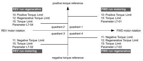
Figure 5.108 Torque Limit Parameters and Analog Input Settings
