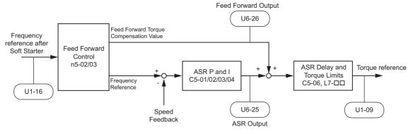
Figure 5.111 Feed Forward Control
