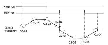
Figure 5.35 S-Curve Timing Diagram - FWD/REV Operation
