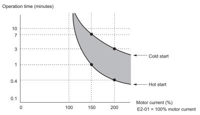
Figure D.9 Motor Overload Protection Time
