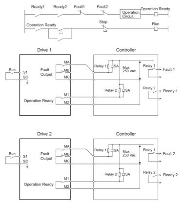
Figure 3.31 Interlock Circuit Example
