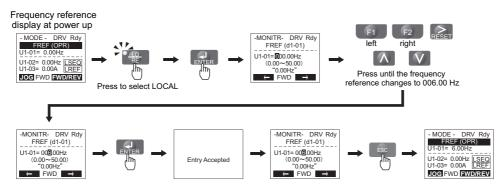
Figure 4.6 Setting the Frequency Reference while in the Drive Mode
