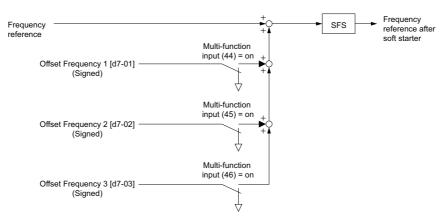
Figure 5.55 Offset Frequency Operation
