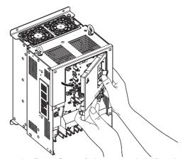
Figure 3.15 Remove the Front Cover (2A0110 to 2A0415 and 4A0058 to 4A1200)
