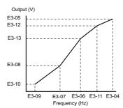
Figure 5.57 V/f Pattern for Motor 2
