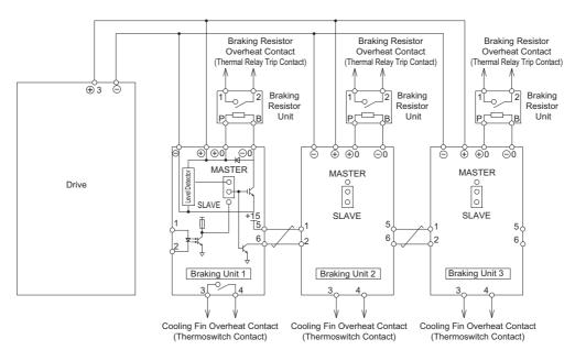
Figure 8.22 Connecting Braking Units in Parallel
