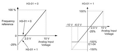
Figure 5.82 Frequency Reference Setting by Analog Input with Negative Bias
