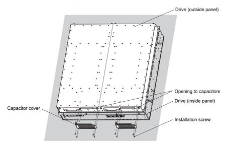
Figure D.11 Capacitor Cover (4A0930, 4A1200)
