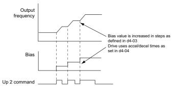
Figure 5.52 Up/Down 2 Bias when  $d4-03 \neq 0.00 \text{ Hz}$
