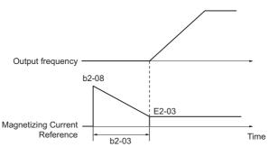
Figure 5.19 Magnetic Flux Compensation
