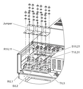
Figure 3.2 Removing the jumper
