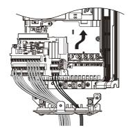
Figure 7.61 Drive Replacement: Installing the Terminal Board
