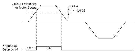
Figure 5.77 Frequency Detection 4 Example with Positive L3-04 Value
