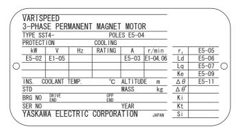
Figure 4.16 Example of Motor Nameplate
