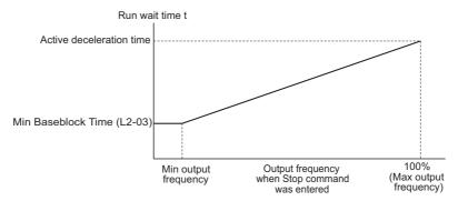
Figure 5.10 Run Wait Time Depending on Output Frequency
