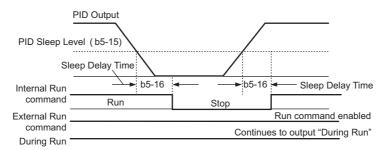
Figure 5.28 PID Sleep Operation
