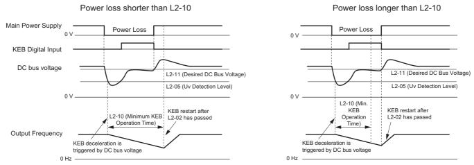
Figure 5.99 KEB Operation Using L2-10 and KEB Input
