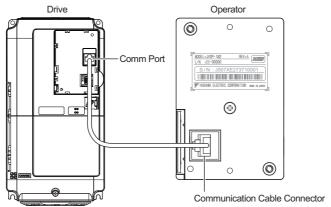
Figure 2.9 Communication Cable Connection
