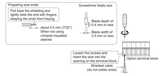
Figure 8.7 Preparing and Connecting Cable Wiring
