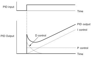
Figure 5.25 PID Operation
