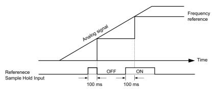
Figure 5.65 Analog Frequency Reference Sample/Hold
