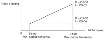
Figure 5.40 ASR Gain and Integral Time in V/fw/PG
