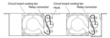
Figure 7.40 Cooling Fan Wiring: 4A0515 and 4A0675
