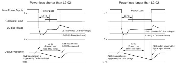
Figure 5.97 KEB Operation Using L2-02 and KEB Input
