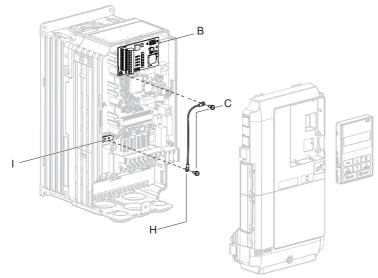
Figure 8.5 Connect the Ground Wire
