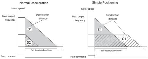
Figure 5.11 Simple Positioning Deceleration
