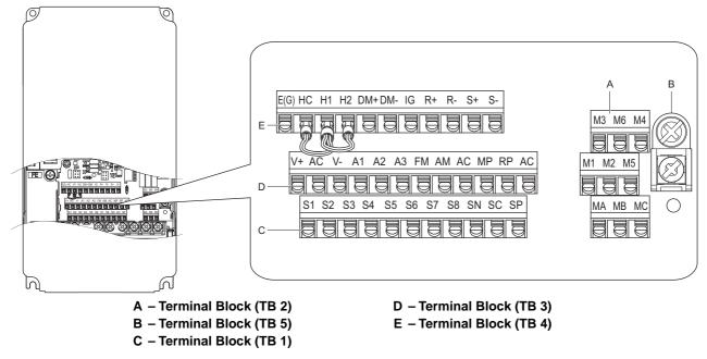
Figure 3.22 Control Circuit Terminal Arrangement
