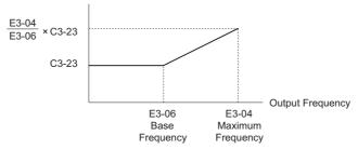
Figure 5.37 Slip Compensation Limit
