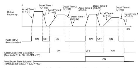
Figure 5.33 Timing Diagram of Accel/Decel Time Change
