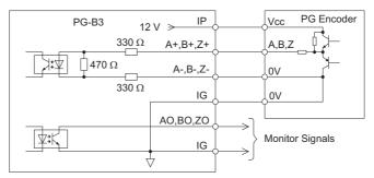
Figure 8.9 Complementary Outputs for the Interface Circuit
