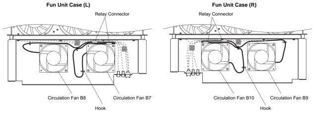
Figure 7.48 Cooling Fan Wiring: Models 4A0930 and 4A1200
