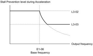
Figure 5.103 Stall Prevention Level and Limit During Acceleration
