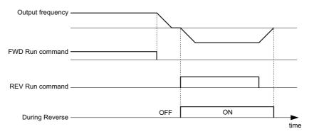
Figure 5.78 Reverse Direction Output Example Time Chart
