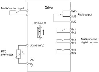
Figure 5.91 Connection of a Motor PTC
