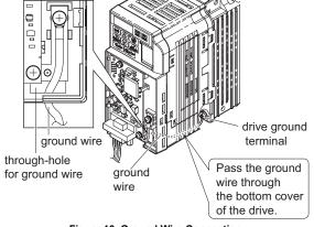
Figure 10 Ground Wire Connection
