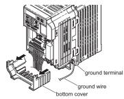
Figure 6 Connect Ground Wire
