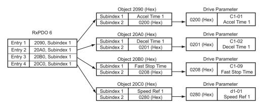
If the PDO contains invalid data, then only the valid data will be written to the drive. Using the example above, if the data for C1-01, C1-09 and d1-01 are valid and the data for C1-02 is out of range, then only parameters C1-01, C1-09 and d1-01 will be changed in the drive, and the data for C1-02 will be ignored.
