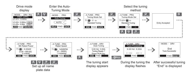
If Auto-Tuning can not be performed for some reason (no-load operation impossible etc.), then set up the maximum frequency and voltage in the E1- $\square$  parameters and enter the motor data manually into the E2- $\square$  parameters.
