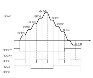
$\ast 1.$  Forward operation at the jog speed is performed while the /JOGP signal is ON.
