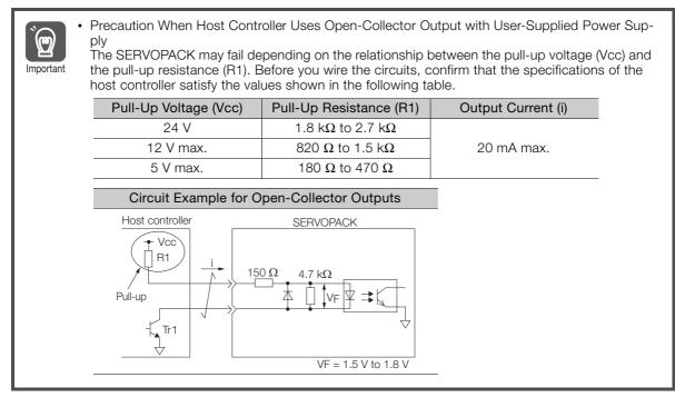
This section describes CN1 connector terminals 40 to 47. The circuits are connected through relay or open-collector transistor circuits. If you connect through a relay, use a low-current relay. If you do not use a low-current relay, a faulty contact may result.
