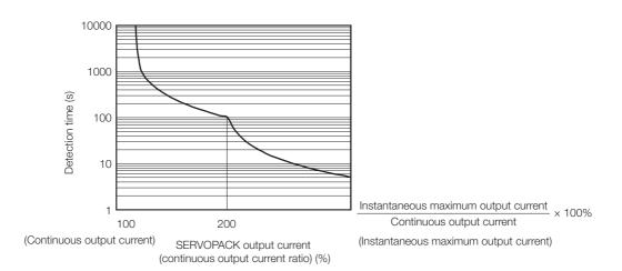
Note: The above overload protection characteristics do not mean that you can perform continuous duty operation with an output of 100% or higher.
