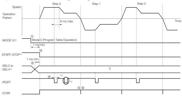
\*1. Do not change /SEL0 to /SEL7 for 4 ms after turning ON the /START-STOP signal.
