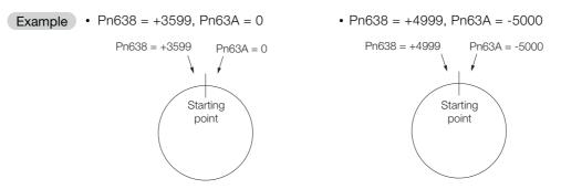
If a rotary table or other device with rotational coordinates is used, but multiturn operation is not possible, use linear coordinates (Pn637 =  $n.\square\square\square$ ). In this case, Pn638 and Pn63A are for software limits.
