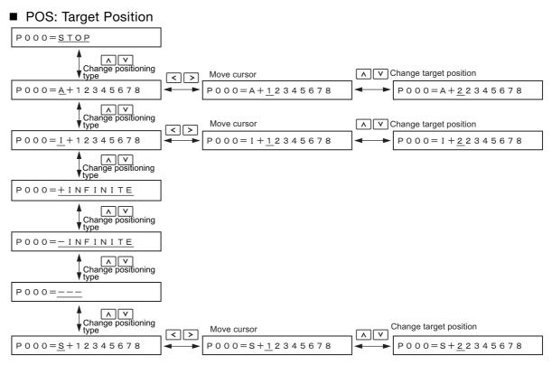
Note: Refer to the following section for details on positioning types and target positions.
