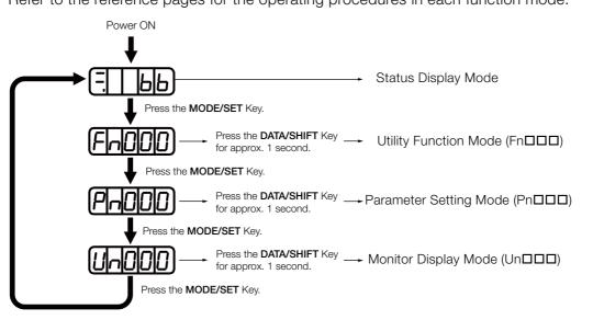
Information You can change the setting of Pn52F (Monitor Display at Startup) to display the Monitor Display Mode instead of the Status Display Mode after the power supply is turned ON. Set Pn52F to the Un number of the monitor display to display after the power supply is turned ON.
