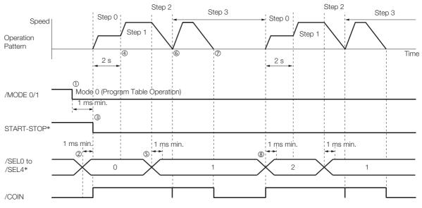
\* Do not change /SEL0 to /SEL7 for 4 ms after turning ON the /START-STOP signal.
