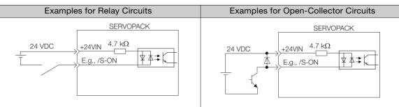
Note: The 24-VDC external power supply capacity must be 50 mA minimum.
