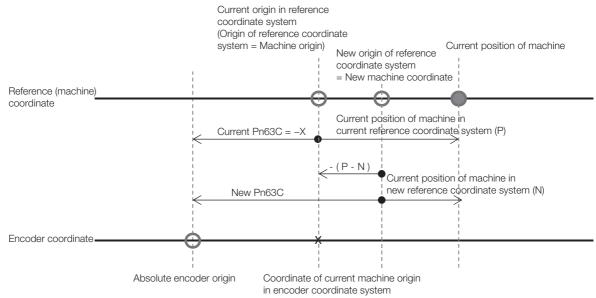
When using the linear type coordinate (Pn637 =  $n.\Box\Box\Box$ ), set the calculated value in Pn63C.
