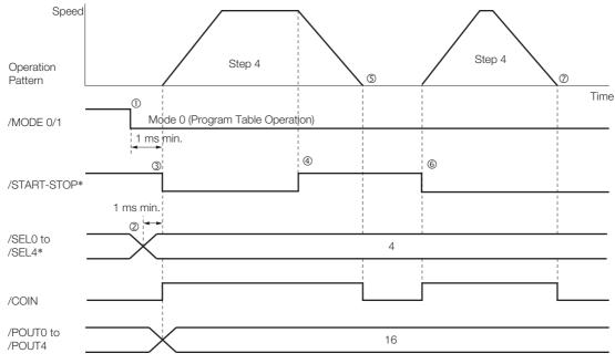
As described below, operation is restarted even when the /START-STOP signal is turned ON even during deceleration after the /START-STOP signal is turned OFF.
