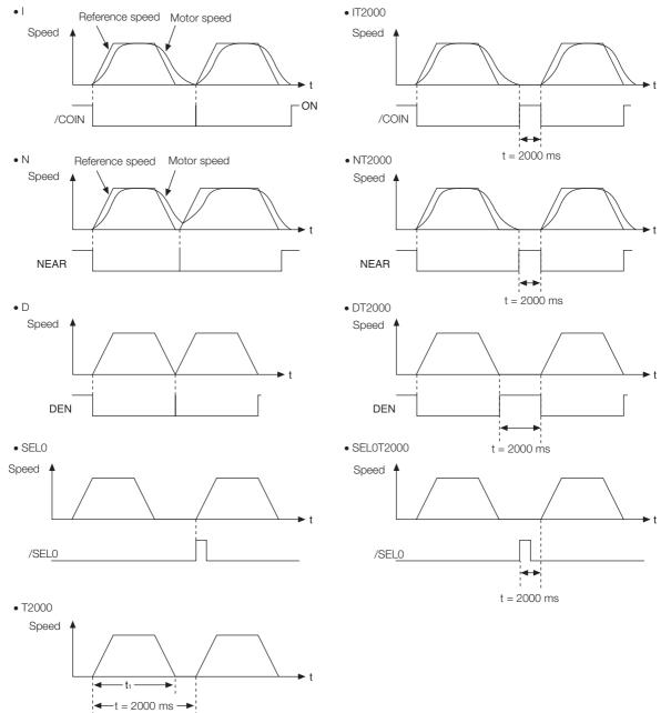
Note: If  $t < t_1$ , an error (E53E) will occur and program table operation will be stopped.
