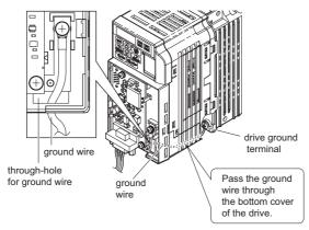
Figure 12 Ground Wire Connection
