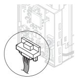
Figure 3 Communication connector location
