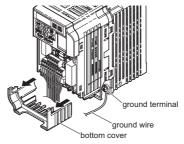
Figure 8 Connect Ground Wire
