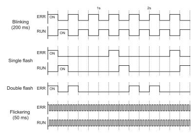
Figure 4 LED Flash Rates and Meaning
