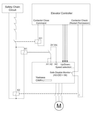
**Note:** 1. The drive output will immediately shut off when either of the inputs H1 or H2 is opened. In this case the brake should apply immediately in order to prevent uncontrolled movement of the elevator.
