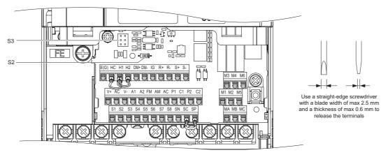
DIP switch S2 and jumper S3 are located on the terminal board. Set them as described below.
