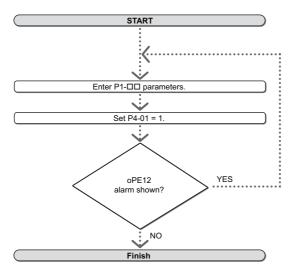
Perform as following to provide the basic parameters:
