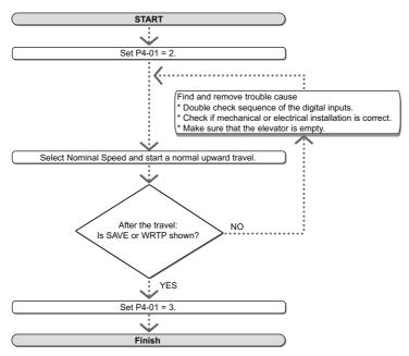
The second teaching step is Empty Car Teach Run. Before doing this step make sure that Basic Calculations teaching has been done successfully and that the distance between switches in the shaft allows at least 1 second leveling travel.
