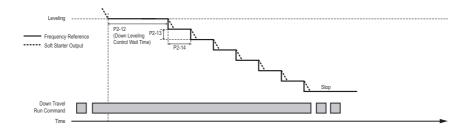
In case the Down Travel RUN command is switched off before reaching zero value, the drive decelerates with Dwell at Stop, if the frequency is still above Stop Dwell level. Refer to the figure below.
