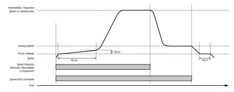
Speeds must be set so that Nominal Speed > Intermediate Speed > Inspection Speed > Leveling Speed. The speeds are set as m/s values in parameters P1-16 to P1-19. These values are calculated for P3-01 to P3-04 as frequency references and must keep the rule P3-01 > P3-02 > P3-03 > P3-04. Not keeping this rule will cause oPE12 alarm. Correct settings and repeat teaching function.
