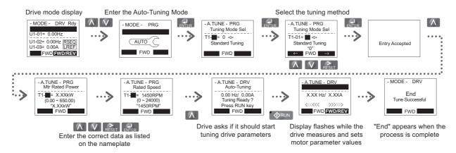
If Auto-Tuning cannot be performed for some reason (no-load operation impossible, etc.), then set the maximum frequency and voltage in the E1- $\square\square$  parameters and enter the motor data manually into the E2- $\square\square$  parameters. Refer to *Auto-Tuning Errors on page 41*.
