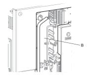
B – Use the open space provided inside the drive to route option card wiring.
