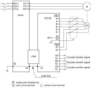
Figure 5 Wiring the Option Card and PG
