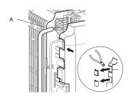
A - Wires should pass through the access hold provided on the left side of the front cover.
