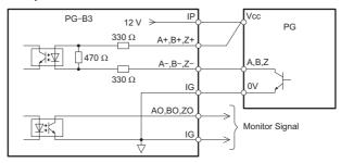
Figure 7 Open-Collector Outputs for the Interface Circuit
