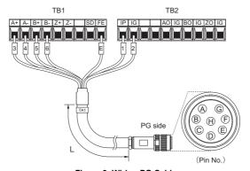
Figure 9 Wiring PG Cables
