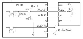
Figure 6 Complementary Outputs for the Interface Circuit
