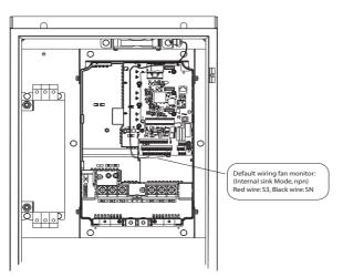
When the A1000 IP54 is operated with control signals other than default (Sink Mode, internal power supply), the fan monitor wiring has to be changed accordingly to following table.
