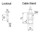
Cable Gland for Control wiring (plastic)
