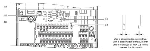
There are three DIP switches and two jumpers, S1 to S5, located on the terminal board.
