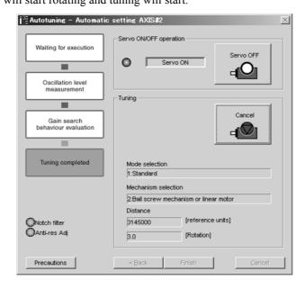
Vibration generated during tuning is automatically detected, and the optimum setting for the detected vibration will be made. When the setting is complete, the LED indicator lamps (bottom left of the box) of the functions used for the setting will light up.
