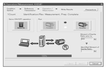
**9.** Click **Reverse** to take measurements by turning (moving) the motor in reverse. After the measurements and the data transmission are finished, the following window will appear.
