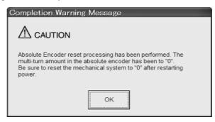
If the encoder is set up successfully, a warning message will appear reminding you that the coordinate system has changed and must also be reset.
